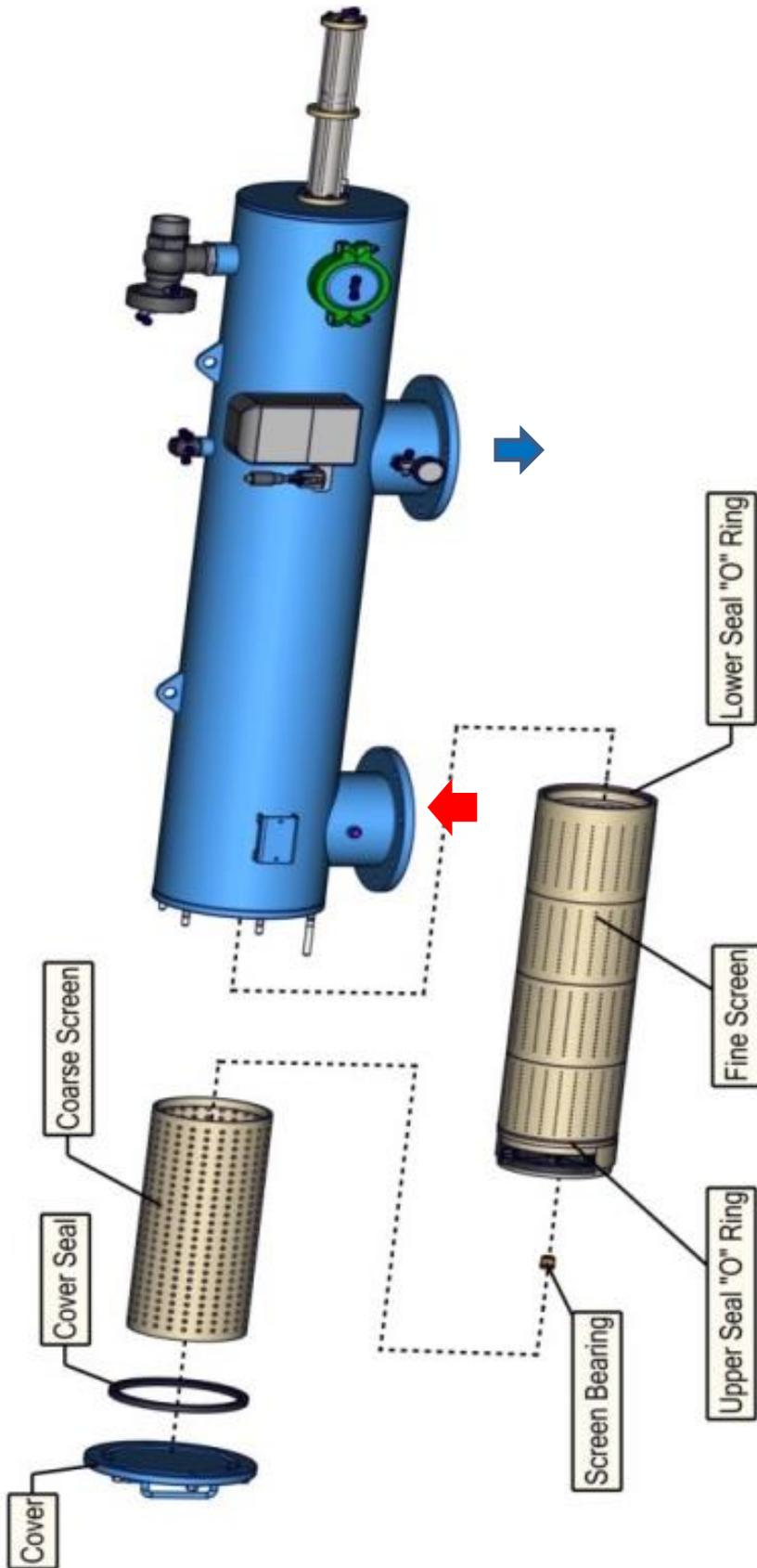
Figure 7: Fine Screen Assembly Removal & Installation
