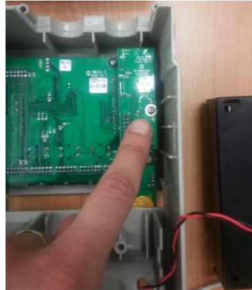
6. Unscrew the main card – 4 screws (Red circles). Remove the card.
