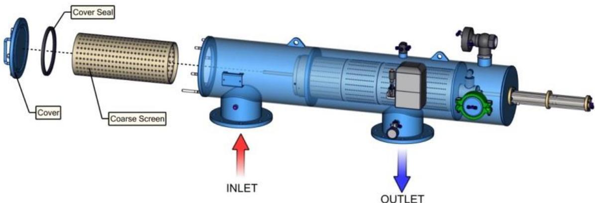
Figure 7: Coarse Screen Removal & Installation
