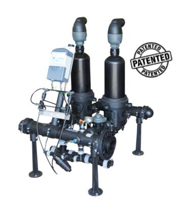
The filter element is composed of highly accurate grooved discs from excellent quality plastic materials. The grooved discs are compressed together to form the filtration element. The intersections between the grooves and the outer surface of the element offer large effective filtration surface with in depth area used to stop debris is especially effective in filtration of organic matter.
